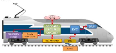
Fig 1- Schematic placement of the OBA on the train. There is no BTM interference
